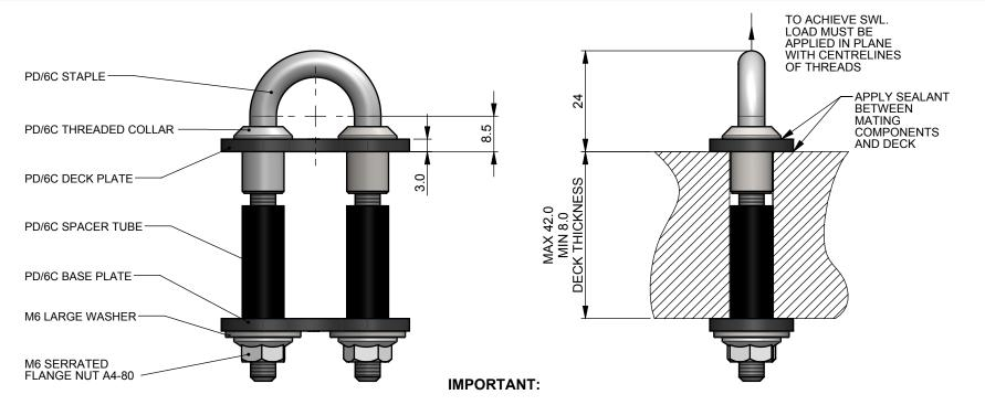
ENSURE PLASTIC SPACER TUBES PROTRUDE THROUGH UNDERSIDE OF DECK AND INTO BASE PLATE HOLES. IF REQUIRED, CUT PLASTIC SPACER TUBES TO LENGTH.
